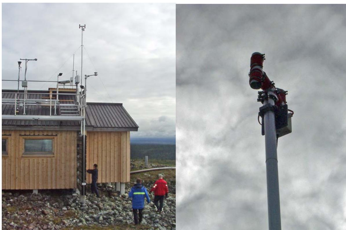
Aerosol is sampled using a custom made, heated inlet approximately 4 meters above the roof of the shelter. This inlet is a acceptable compromise to avoid clogging of the inlet during cloud and snow periods. The estimated cut-off size is 7  $\mu\text{m}$ . The influence of wind-direction on the sampling efficiency of this inlet has not been tested. Due to the asymmetric design it is, however, probably not omni-directional. Sample flow inside the sampling tube is turbulent.
