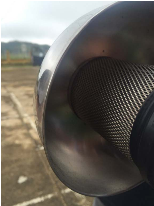
Actual TSP inlet, showing the insect screen
