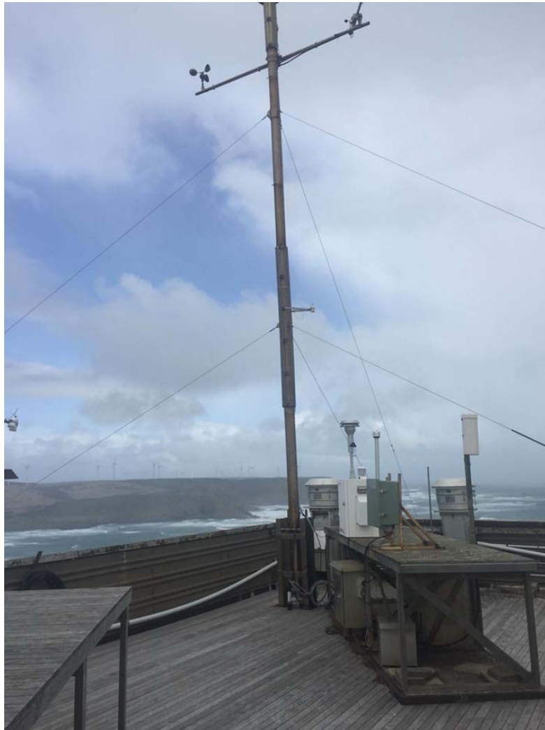
Figure 2: main aerosol inlet of Cape Grim.
