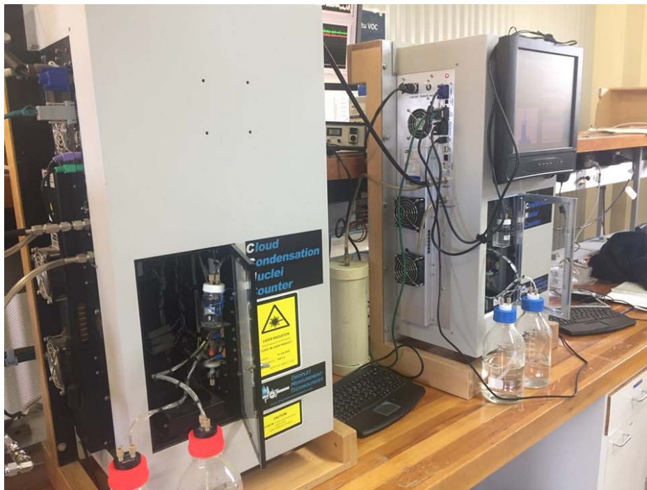
Figure 12: Set-up of the two DMT CCN counters.
