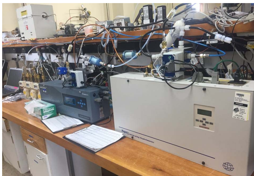
Figure 4: Set-up of the two Ecotech integrating nephelometers.
