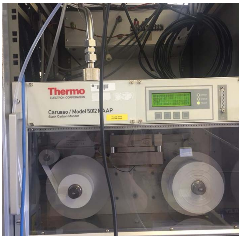
Figure 8: Multi-Angle Absorption Photometer
