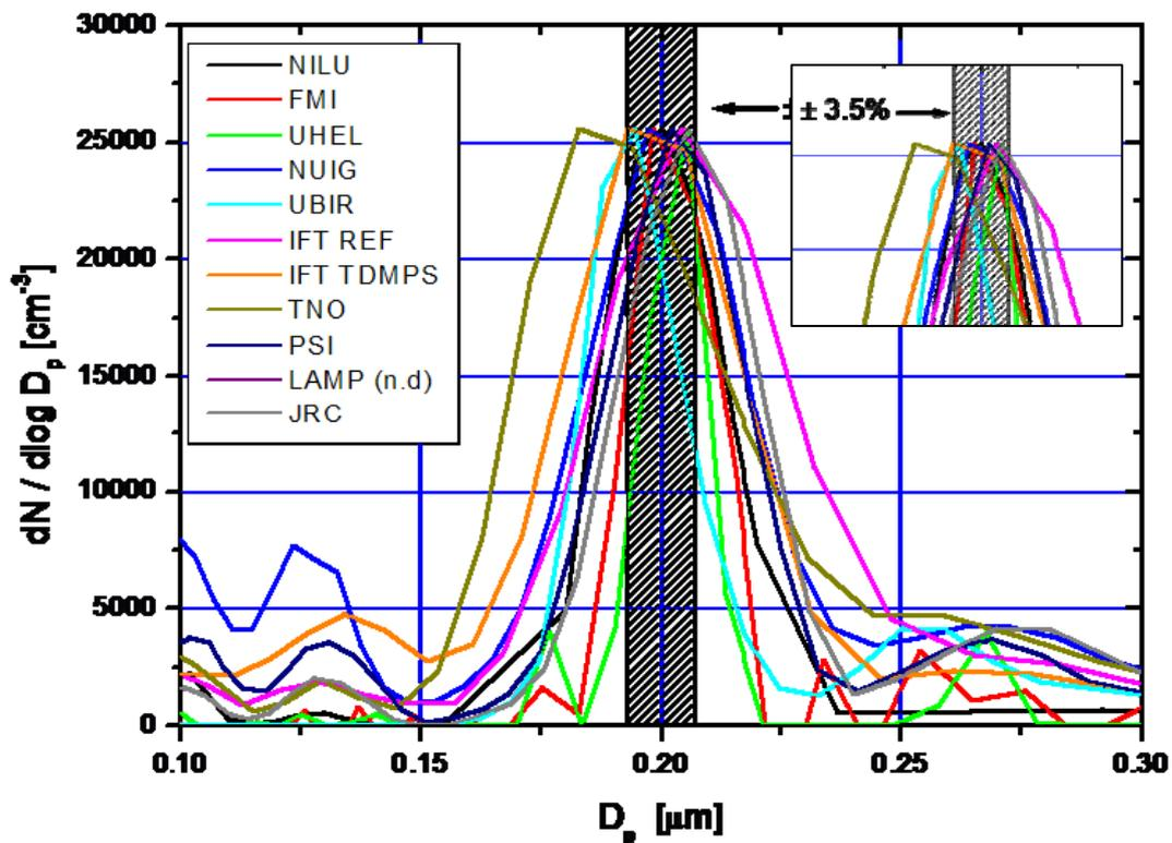
Fig 2: Latex Nanospheres at 200 nm, normalized to maximum of particle number of SMPS reference system, grey colored area shows  $\pm 3.5\%$  variation of diameter shift of SMPS reference system
