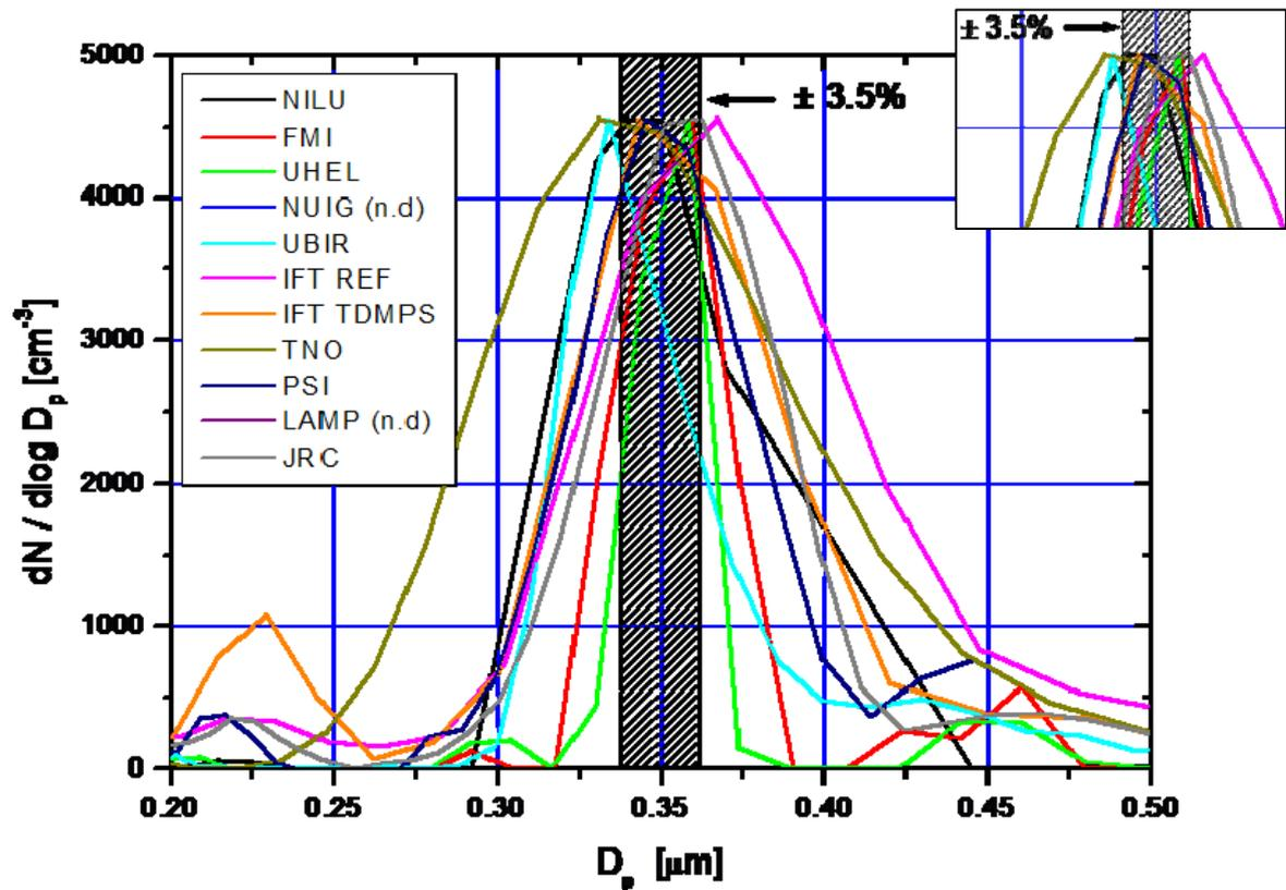
Fig 3: Latex Nanospheres at 350 nm, normalized to maximum of particle number of SMPS reference system, grey colored area shows  $\pm 3.5\%$  variation of diameter shift of SMPS reference system
