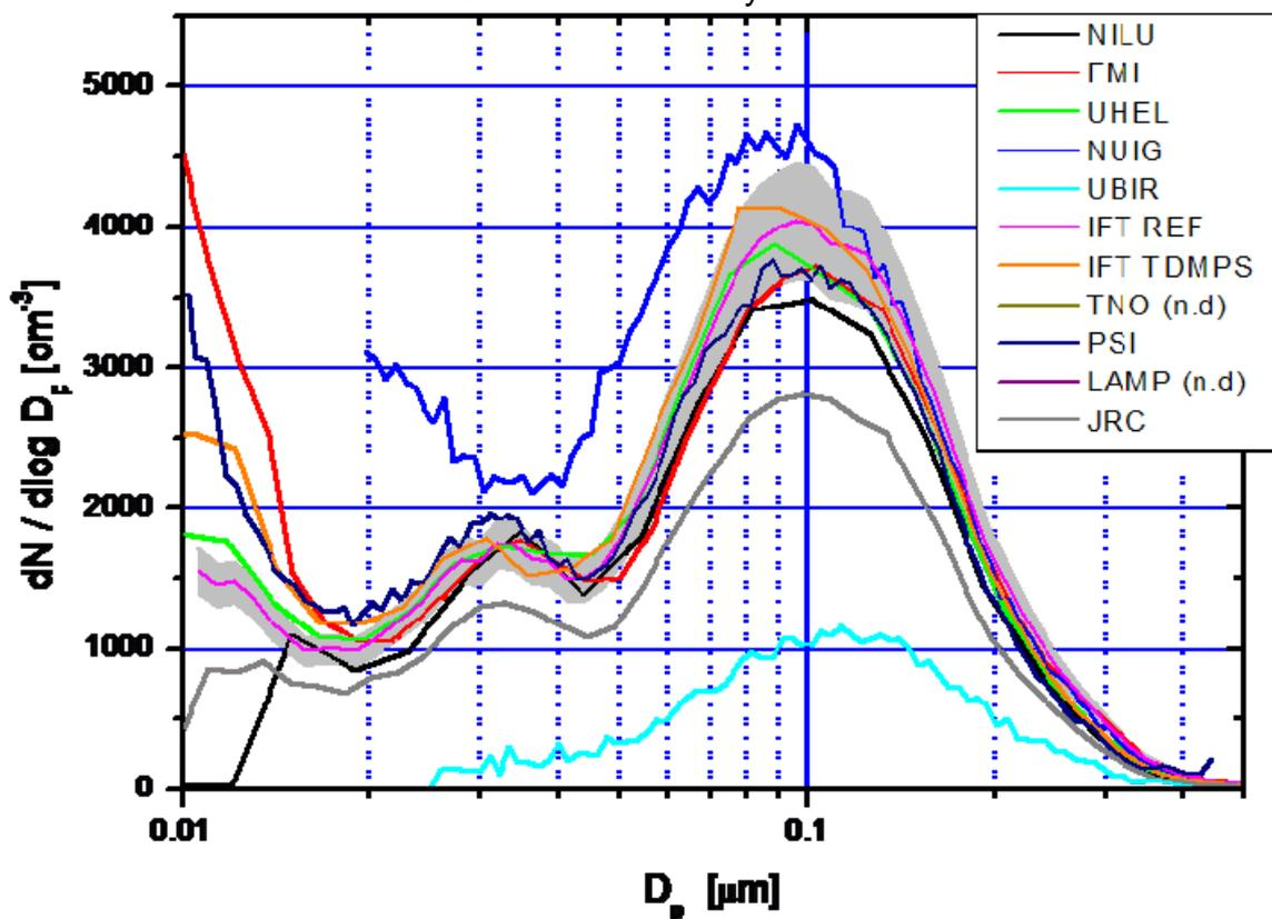
Fig 4: Particle number size distributions for an ambient aerosol, grey colored area shows  $\pm 10\%$  variation of concentration of SMPS reference system.
