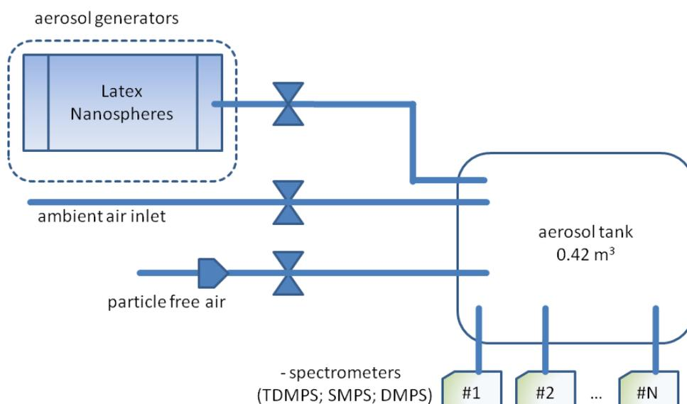
Fig 1: Schematic scheme of calibration setup for spectrometer workshop.
