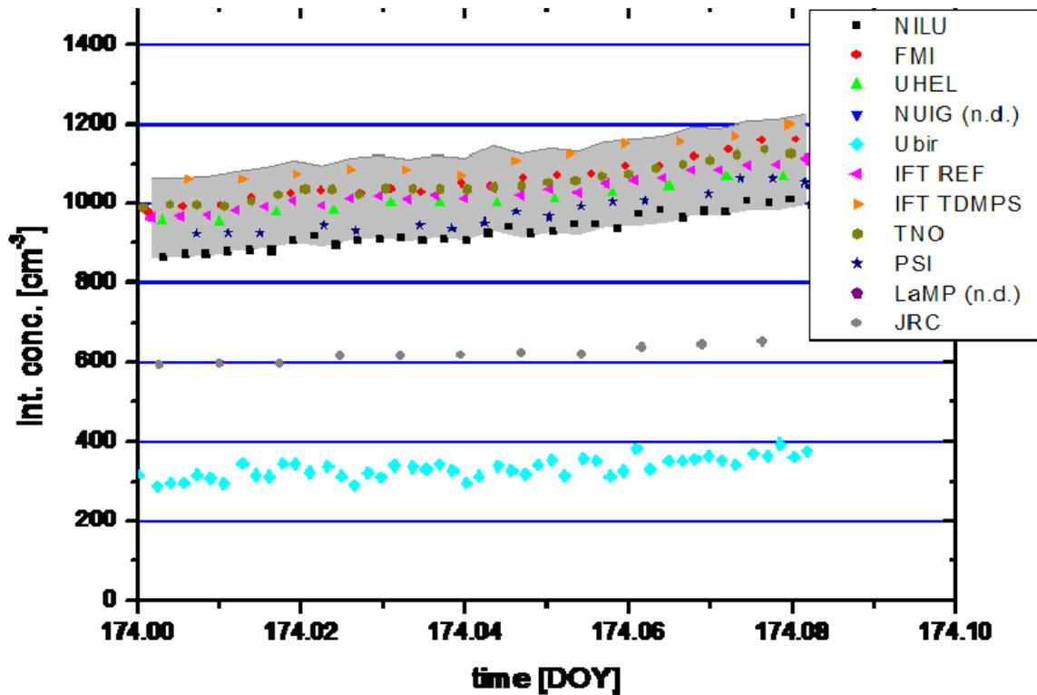
Fig 6: Absolute concentration > 100 nm, corrected for losses by each operator, grey colored area shows  $\pm 10\%$  variation of concentration of SMPS reference system.
