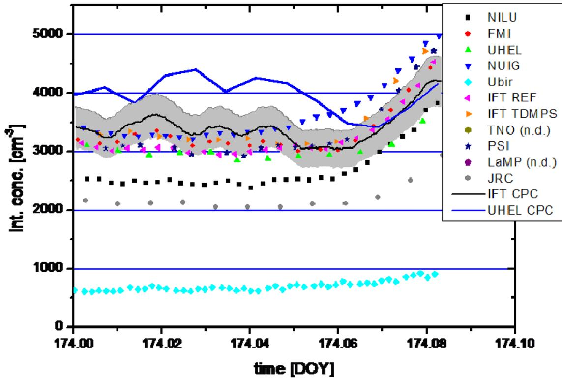
Fig 5: Absolute concentration for particle > 10nm, corrected for losses by each operator, grey colored area shows  $\pm 10\%$  variation of concentration of SMPS reference system.
