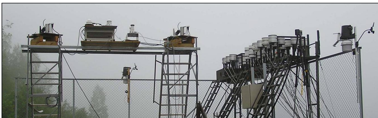
Figure 1. Solar platform at the roof of NRPA during the core period of the intercomparison. Front section: Eppley TUVR and Solar Light broadband meters flanked by two rotating shadowband MBFRs. Right section: NILU-UVs, GUVs and the front optics of 4 Bentham spectroradiometers. In the background and to the far right: Davis automated weather stations. ( Photo: G. Janson, USDA ).
